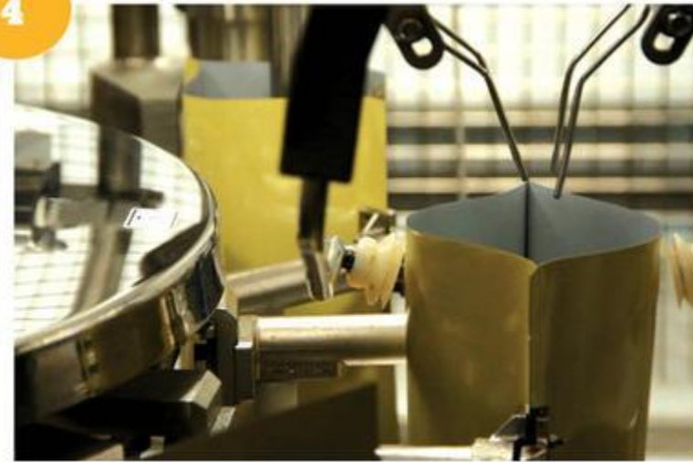
The Pouches are then nitrogen flushed. This removes any oxygen ensuring the pouch is sterile and the flavour of the malt extract is retained.
