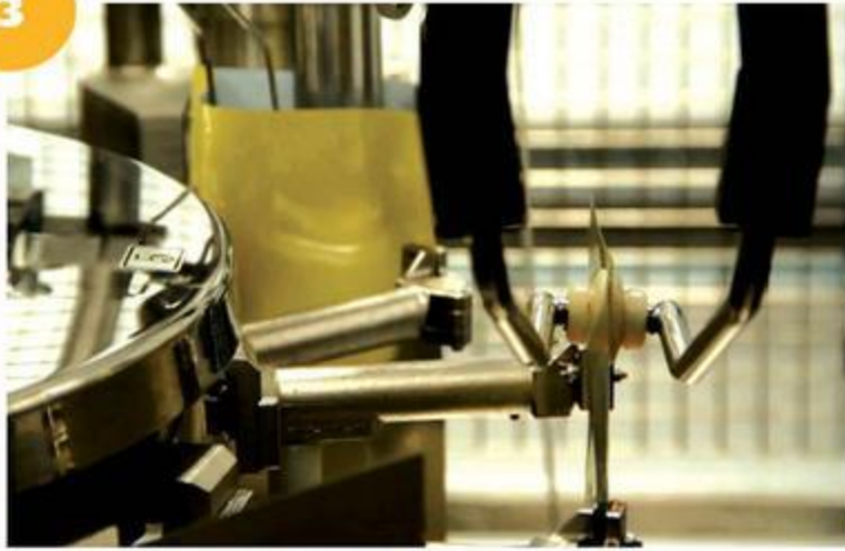
Pouches opened using air suction.
